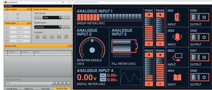
Design Studio includes a 'Preview in Emulator' function which emulates the hardware inputs/outputs allowing you to test projects prior to their upload to the PanelPilotACE display via USB.
